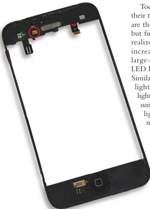
FIGURE 1. Light and proximity sensors are often located next to a handheld device's speaker because both the sensors and the speaker require access to the outside world. The proximity sensor in a 3G iPhone is within the red circle, and the ambient-light sensor is the green part to its left. The iPhone's speaker is the gray, mesh-colored oblong. (See "iPhone puts proximity detection in your face," p. 52.) Courtesy of iFixit.
